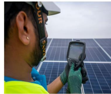
Figure 8: Thermal inspection through thermal imaging camera
